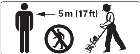
Within a wide area around the workplace, there is a risk of accident by ejected objects, therefore ensure that there is no-one within a 5 m radius of the machine. This distance must also be maintained in relation to objects (vehicles, window panes) – **risk of property damage!** Even at a distance over 5 m, danger cannot be ruled out.
